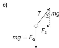
$$\sin \varphi = F_z/T, \cos \varphi = mg/T \Rightarrow F_z/(\sin \varphi) = mg/(\cos \varphi)$$
